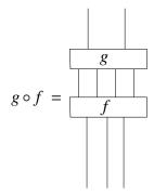
In this diagram we have omitted the boundary box, fixed points and string labels as explained in Definition 5. It is important to note that two string diagrams can be composed only when the fixed points and string labels match in the middle. This is equivalent to saying that  $g \circ f$  is defined only when the domain of g equals the codomain of f. For string diagrams, tensor product is horizontal stacking:
